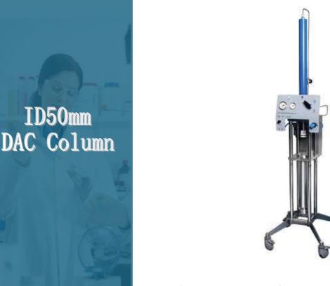
The DAC (dynamic axial compression) column adopts latest design by ATL. The piston of column always produces a stable pressure on packing bed which can effectively prevent the collapse and loose of the column bed.
